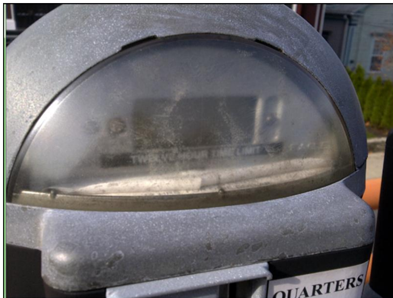
Figure 2-16: Example of the Sup-Par Conditions of Parking Meters
